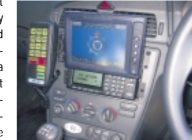
The UK test site used a Sussex police car equipped with this in-vehicle display and interface to visualise the minimum set of data (MSD).
