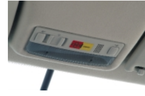
The manual emergency call button for the Seat test vehicle was located above the rear-view mirror.
